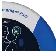
Figure 11. Flashing green LED; no action required.
